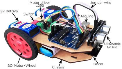
The obtained values from the ultrasonic sensor need to be calibrated in order to get a meaningful data (distance). The distance of the object is calculated on the basis of the time taken by the wave in the process of transmission, reflection and collection.
